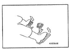
Shift the high/low speed control lever as shown.
