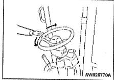
When turning, keep to the inner side when advancing and outer side when reversing, considering the properties of the rear steering system.
