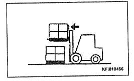
5. Lower the load temporarily to the stacking point.
