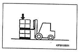
Reverse the lift truck slowly and withdraw the forks fully from beneath the load.
