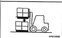
8. Reverse the lift truck to a position where the load can be safely lowered.
