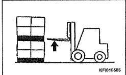
Drive forward and insert the forks 2/3 to 3/4 of the way under the load, then raise the load 2 - 4 in. (5 - 10 cm).
