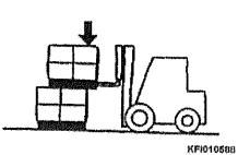
Drive forward slowly and insert the forks fully under the load.
