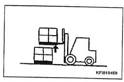
8. Position the load correctly above the stacking point.
