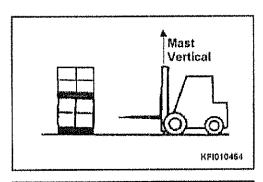
2. Align the forks with the fork insertion point.
