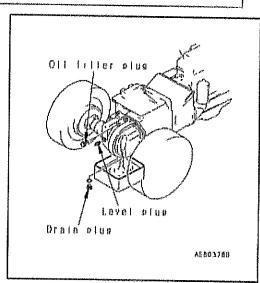
addition to checking and changing the oil in the differential case in two separate operations.
