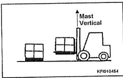
3. Raise the load to 2 - 4 in. (5 - 10 cm) above the stacking point.
