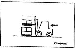
9. Lower the load to the correct stacking position.
