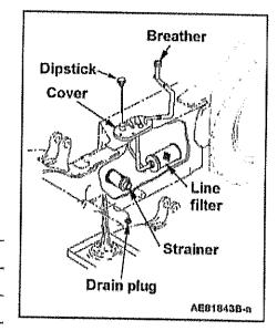
6. Start the engine, then operate the cylinders (lift, tilt) to the end of their travel 5 or 6 times to bleed the air.
