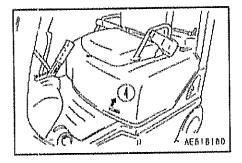
3. Lift the hood all the way up (5) until the engine hood stopper fits into place.
