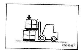
Reverse and slowly withdraw the forks 1/4 to 1/3 of the way out from beneath the load.
